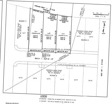
BEARINGS ARE MONUMENTED AND SHOWN BASED UPON THE TWO FOLLOWING CITY OF BROOMFIELD CPS CONTROL POINTS, CPS No. 9 AND CPS NO. JEFFCO AZ MK AS BEING NOS49'04'E, AND A MEASURED DISTANCE OF 8634.54 FEET, AS MONUMENTED AND SHOWN HEREON.
